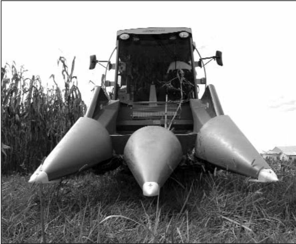
A small plot combine purchased with a grant from the U.S. Department of Energy allows researchers at Southern Illinois University Carbondale to harvest and take data from a strip of field just two rows wide. Photo by Russell D. Bailey
